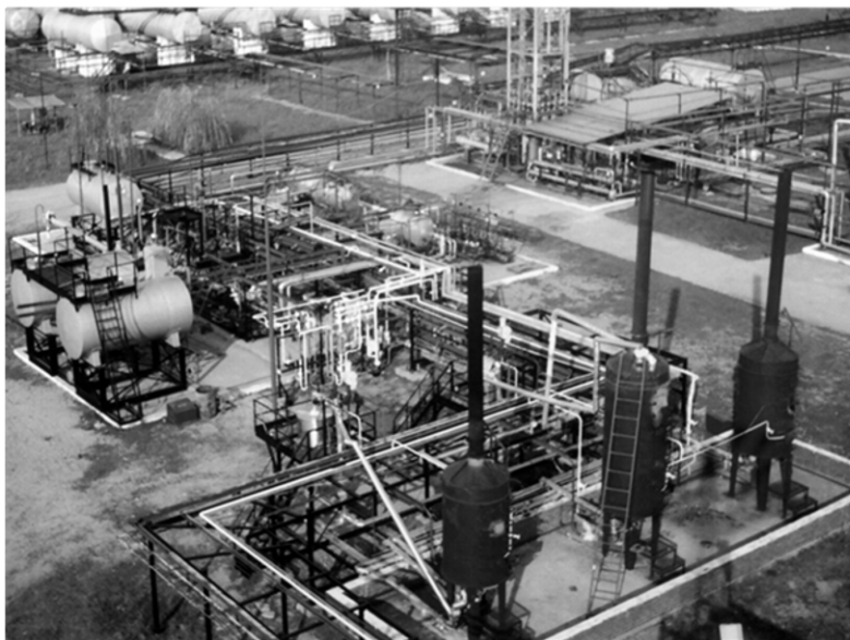
Fig. 3. A semicommercial installation for associated gas aromatization ( C_2 – C_4 hydrocarbons) with the capacity of 1000 ton year -1 (Krasnodar).
